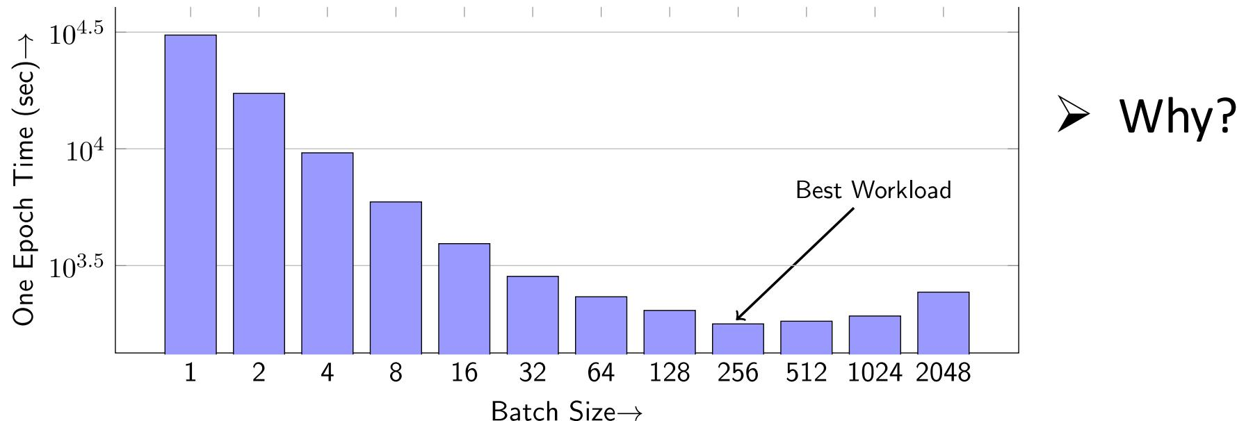
One epoch training time of AlexNet computed on an Intel KNL system
