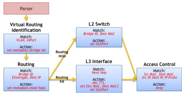
Figure 3: Table dependency graph for an L2/L3 switch.
