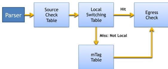
Figure 4: Flow chart for the `mTag` example.
